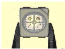
(3) When populating boards in SMT production, there are basically no restrictions regarding the form of the pick and place nozzle, except that mechanical pressure on the surface of the resin must be prevented.
