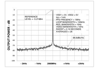
Fig. 15 AK1545 Phase Noise (2800 MHz, 1 MHz, 100 kHz)
