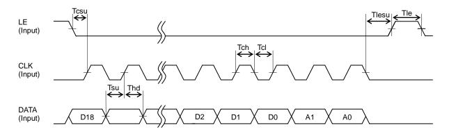
Fig. 3 Serial Interface Timing Chart
