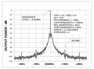
Fig. 17 AK1545Reference Spurs (2800 MHz, 1 MHz, 100 kHz)
