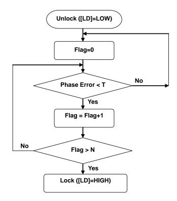
Fig. 8 Unlocked  $\rightarrow$  Locked
