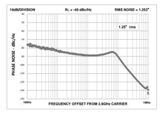
Fig. 16 AK1545 Integrated Phase Noise (2800 MHz,
