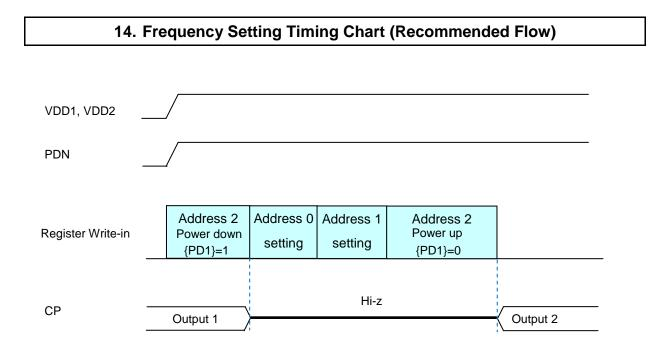
Fig. 12 Frequency settings (controlled by {PD1})
