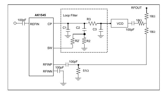
Fig. 34 Typical Evaluation Board Schematic
