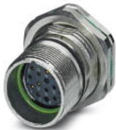
Device connector for rear wall, straight, shielded: yes, SPEEDCON locking, M23, No. of pos.: 16+2+PE, type of contact: Socket, Crimp connection, Axial seal, Central fixing
