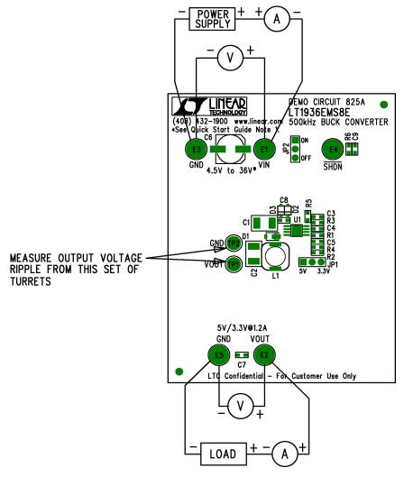
Figure 1. Proper Measurement Equipment Setup
