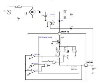
Figure 5. Start-up circuit block diagram
