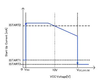
Figure 6. Start-up current-VCC voltage curve
