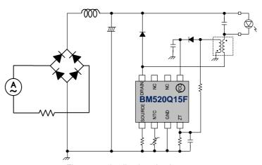
Figure 1. Application circuit
