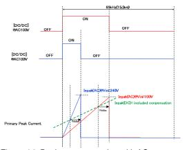
Figure 13. Peak current sensing without AC compensation
