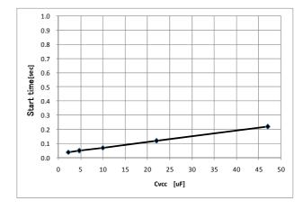
Figure 7. Start-up time – VCC capacitance characteristics
