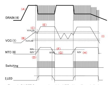
Figure 9. ON/OFF Sequences (supplying VCC with auxiliary winding)
