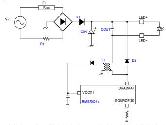
Figure 8. Schematic of the DC/DC Part while Supplying with the Auxiliary Winding
