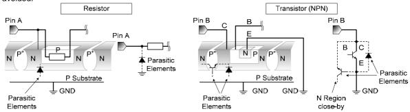
**Example of monolithic IC structure**
