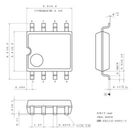
Figure 4. SOP8 package external dimensions
