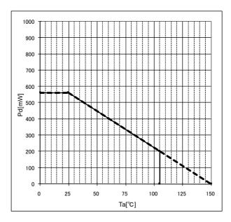
Figure 16. Power Dissipation characteristics
