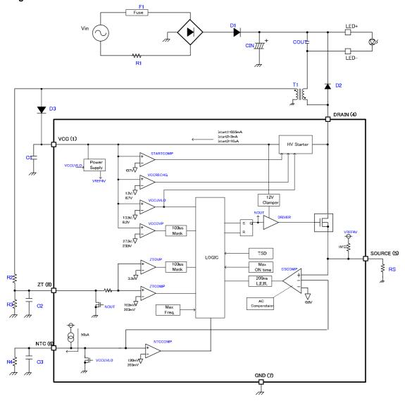
Figure 3. Block diagram
