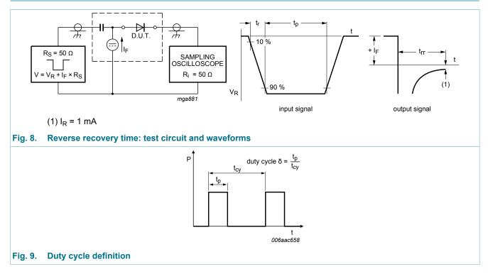
The current ratings for the typical waveforms are calculated according to the equations:  $I_{F(AV)} = I_M \times \delta$  with  $I_M$  defined as peak current,  $I_{RMS} = I_{F(AV)}$  at DC, and  $I_{RMS} = I_M \times \sqrt{\delta}$  with  $I_{RMS}$  defined as RMS current.
