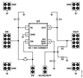
Figure 2. Evaluation Board Schematic
