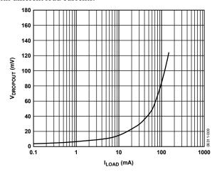
Figure 8. Dropout Voltage vs. Load Current
