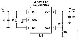
Figure 3. ADP1710 Adjustable Output
