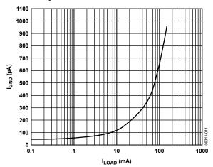
Figure 10. Ground Current vs. Load Current.
