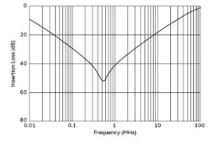
Common Mode Insertion Loss (Typ.)
