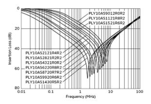
Differential Mode Insertion Loss-Frequency Characteristics
