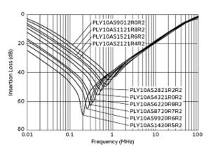
Common Mode Insertion Loss-Frequency Characteristics
