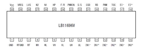
Figure 2. Pin Assignment
