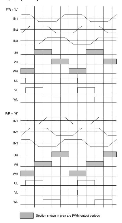
Figure 3. Hall Sensor Signal Input/Output Timing Chart
