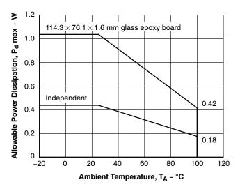
Figure 1. P<sub>d</sub> max – T<sub>A</sub>
