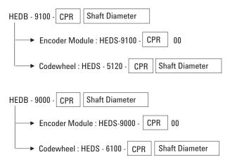
$Note: The \ bundle \ part\ HEDB-9100/9000\ consists\ of\ HEDS-9100/9000\ and\ HEDS-5120/6100. The\ diagram\ below\ provides\ the\ breakdown\ list.$
