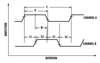
Figure 2. Output waveforms
