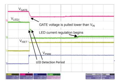
Figure 2: Power Up Diagram Showing Disconnect,  $V_{\rm GATE}, V_{\rm LED1}, V_{\rm ISET}$ , and  $V_{\rm PWM}$  During LED Pins Detect and Regulation Period
