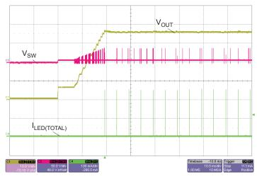
Start up at 0.02% PWM Dimming at 200 Hz, V<sub>IN</sub> = 7 V, 2 Channels, 10 LEDs/Channel, 120 mA/Channel; Time base = 10 ms/Div
