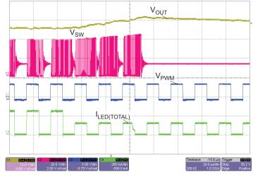
Figure 22: Typical OVP Condition Caused by an Open LED String
