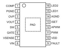
Package LP, 16-Pin TSSOP Pinout Diagram
