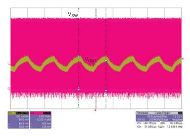
Figure 33: Output Voltage Ripple Frequency Due to Dithering = 12.4 kHz at  $V_{\rm IN}$  = 12 V, and PWM Ratio = 100%
