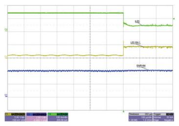
Figure 20: Disabling of LED1 String when the LED1 Pin Voltage is Increased Above 4.6 V
