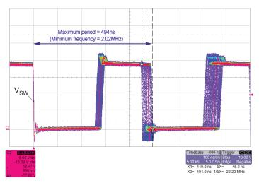
Figure 31: Minimum Dithering Switching Frequency = 2.02 MHz at V<sub>IN</sub> = 12 V, and PWM Ratio = 100%
