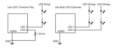
Figure 3: Channel Select Setup
