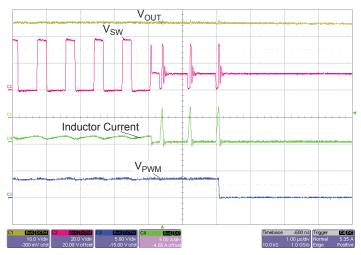
Figure 26: Secondary Boost Switch OCP
