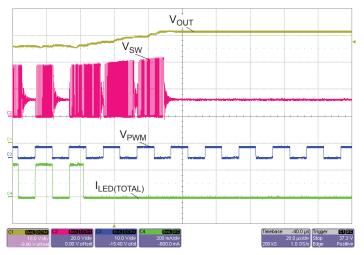
Figure 21: Output of A8518 when Disconnetced from Load During Normal Operation
