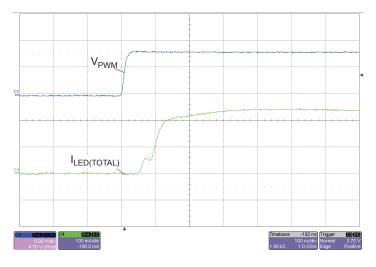
Figure 10: Rising Edge PWM Signal to Total LED Current I<sub>LED(TOTAL)</sub> Turn-On Delay. Time base = 100 ns
