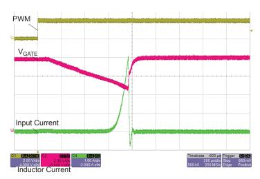
Figure 28: Startup into Output Shorted to GND Fault. Input OCP tripped at 4 A ( $R_{SC}$  = 0.024  $\Omega$ ,  $R_{adi}$  = 383  $\Omega$ )
