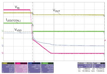
Figure 29: Shutdown with Falling Input Voltage
