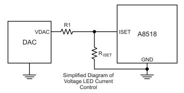
Figure 19: Typical Application Circuit Using a DAC and  $R_{\rm ISET}$  Resistor to Control the LED Current in the A8518
