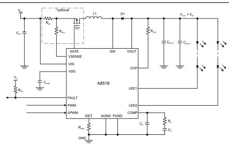
Typical Application Circuit Showing VOUT-to-Ground Short Protection Using Optional P-Channel MOSFET
