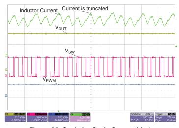
Figure 25: Cycle-by-Cycle Current Limit
