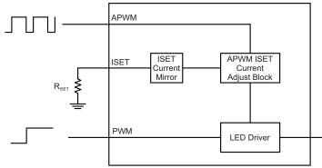
Figure 12: Simplified Block Diagram of APWM ISET
