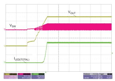
Start up at 100% PWM Dimming,  $V_{IN}$  = 7 V, 2 Channels, 10 LEDs/Channels, 120 mA/Channels; Time base = 10 ms/Div
