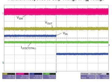
From  $V_{IN}$  = 16 V to  $V_{IN}$  = 5.5 V, 2 Ch, 120 mA/Channel, PWM = 100%; Time base = 20 ms/Div
