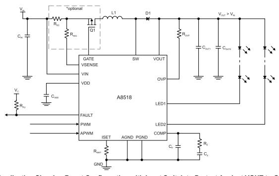
Typical Application Showing Boost Configuration with Input Switch to Protect Against VOUT-to-GND Short
