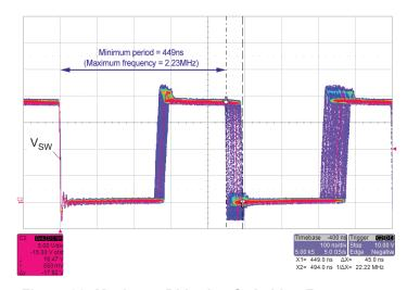
Figure 32: Maximum Dithering Switching Frequency = 2.23 MHz at  $V_{IN}$  = 12 V, and PWM Ratio = 100%
