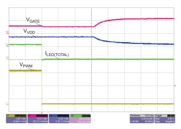
Figure 30: Shutdown Using the Enable
