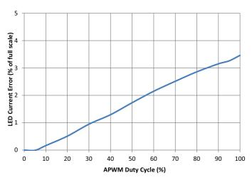
Figure 14: Error in LED Current vs. APWM Duty Cycle  $V_{IN}$  = 9 V,  $V_{OUT}$  = ~22 V,  $R_{ISET}$  = 24 k $\Omega$ , APWM = 200 kHz
