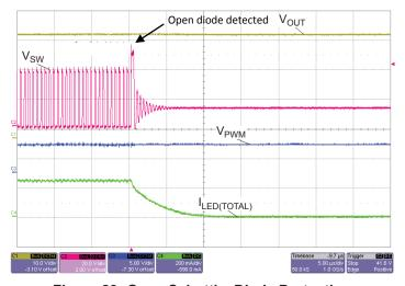
Figure 23: Open Schottky Diode Protection
