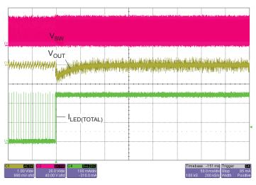
From PWM = 0.1% to PWM = 100% at 120 mA/Channel,  $V_{IN}$  = 12 V; Time base = 50 ms/Div
