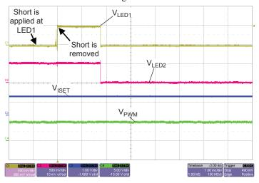
Figure 6: One LED is Shorted to GND.
