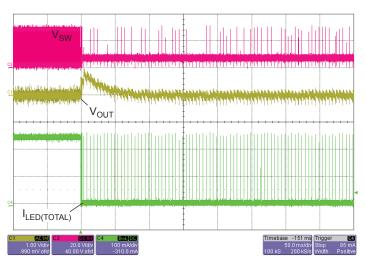
From PWM = 100% to PWM = 0.01% at 120 mA/Channel,  $V_{IN}$  = 12 V; Time base = 50 ms/Div
