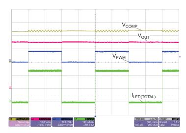
Figure 8: Typical PWM Diagram Showing V<sub>OUT</sub>, I<sub>LED</sub>, and COMP Pins, as well as the PWM Signal. (PWM dimming Frequency is 500 Hz 50% duty cyle.)
