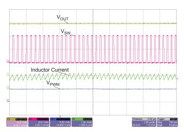
Figure 24: Normal Operation of Switch Node (V<sub>SW</sub>), Inductor Current and Output Voltage (V<sub>OUT</sub>)
