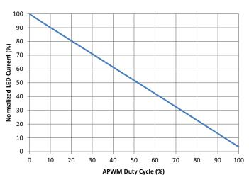
Figure 13: Normalized LED Current vs. APWM Duty Cycle  $V_{IN}$  = 9 V,  $V_{OUT}$  = ~22 V,  $R_{ISET}$  = 24 k $\Omega$ , APWM = 200 kHz
