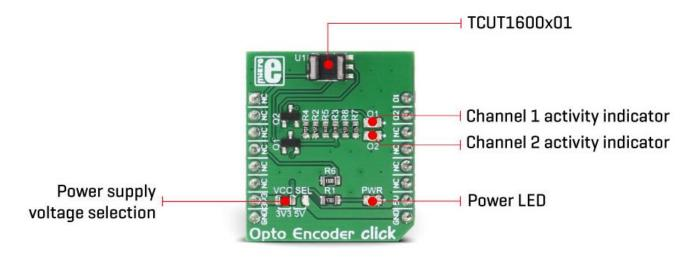
Since the signals of these two output channels are not enough to drive pins on a host MCU, the Click board<sup>™</sup> features two additional MOSFETs. These MOSFETs are also used to drive two additional LEDs, which indicate activity of each channel. E1 and E2 pins are routed to the MOSFET gate pins, while the MOSFET drains are routed to the mikroBUS<sup>™</sup> PWM and INT pins. These pins are pulled to a LOW logic level by the pull-down resistors, to avoid floating.
