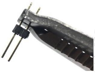
For this next step, a pair of pliers is handy. First, grab the 6 header pins all attached together and break them into 3 sets of 2 header pins. Then, grab them in the pliers like shown here, and then slightly bend them so they look like the next picture.
