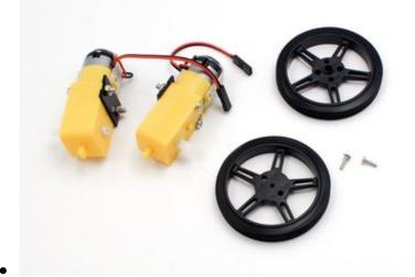
Take the two wheels, rubber treads, and 2x small screws found in the same bag as the wheels.
