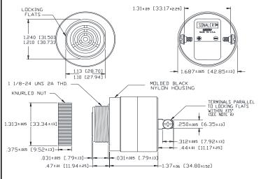
NOTE A: TERMINALS-032 BRASS TIN PLATED, TAPPED FOR #6-32 SCREW. TWO #6-32 NICKEL PLATED BRASS SCREWS INCLUBED. WILL ACCEPT 1/4\* QUICK CONNECT.
