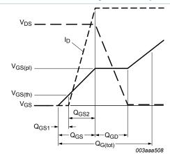
Fig. 13. Gate charge waveform definitions
