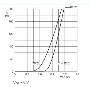
function of source-drain (diode forward) voltage; typical values
