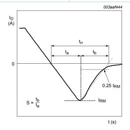
Fig. 16. Reverse recovery timing definition
