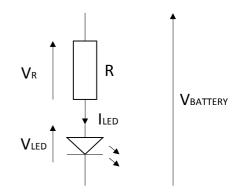
Using Ohms Law in a slightly rearranged format:
