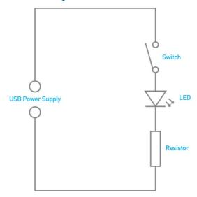
The circuit diagram for the USB lamp is shown above. It is a very simple circuit. The 5V that powers the circuit is supplied from the micro USB connector.
