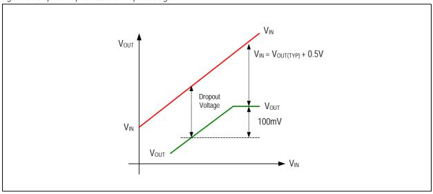
Figure 15 shows the variation of Vout as VIN is varied for a certain load current. The practical value of dropout is the differential voltage (Vout-VIN) measured at the point where the LDO output voltage has fallen by 100mV below the nominal, fully regulated output value. The nominal regulated output voltage of the LDO is that obtained when there is 500mV (or greater) input-output voltage differential.
