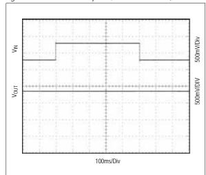
Figure 10. Load Transient Response; IOUT = 0mA to 100mA
