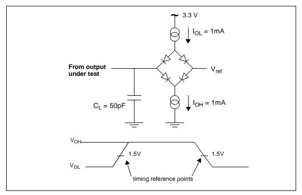
Figure 12 Output load circuit waveform
