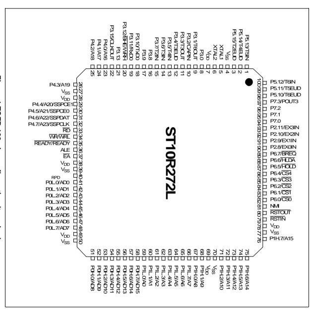
Figure 1 TQFP-100 pin configuration (top view)
