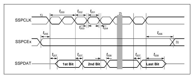
Figure 29 SSP write timing
