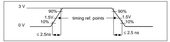
Figure 11 Input waveforms
