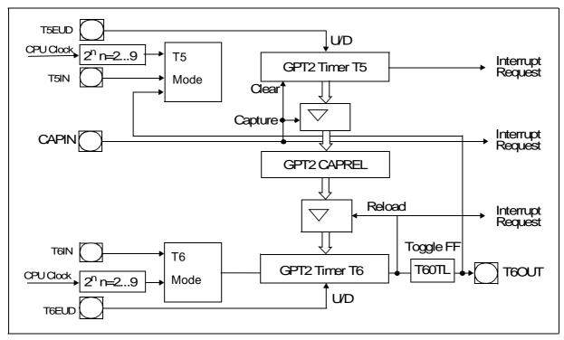
Figure 9 GPT2 block diagram
