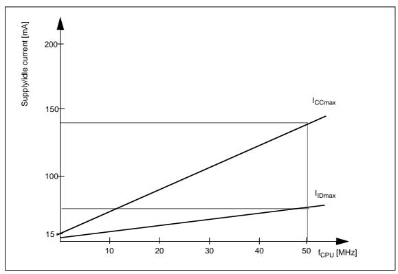
Figure 10 Supply/idle current vs operating frequency
