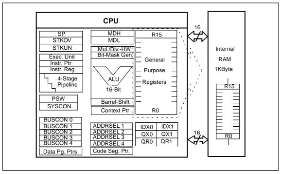
Figure 4 CPU block diagram
