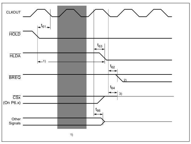
Figure 25 External bus arbitration, releasing the bus
