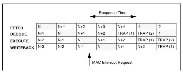
Figure 7 Pipeline diagram for MAC interrupt response time
