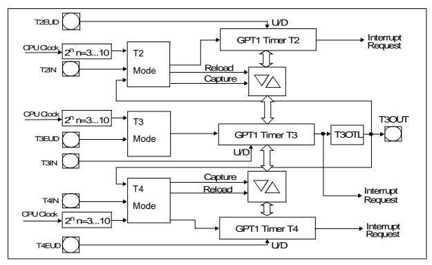
Figure 8 GPT1 block diagram
