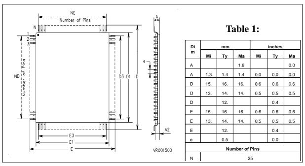
Figure 31 Package outline TQFP100 (14 x 14 mm)
