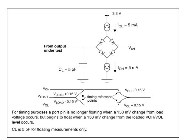
Figure 13 Float waveforms
