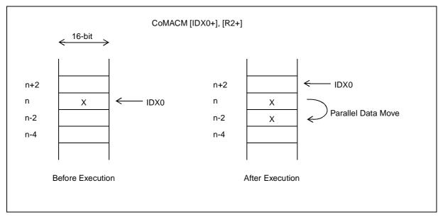
Figure 6 Example of parallel data move
