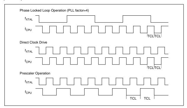
Figure 14 CPU clock generation mechanisms
