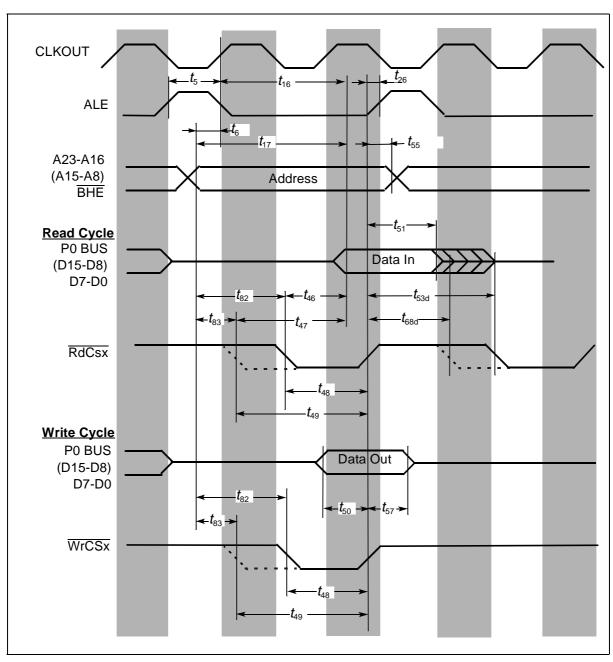
Figure 22 External memory cycle: demultiplexed bus, with/without read/write delay, normal ALE, read/write chip select
