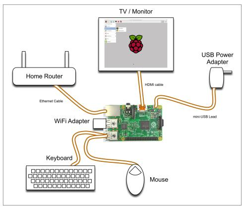
Figure 1-6. A typical Raspberry Pi system
