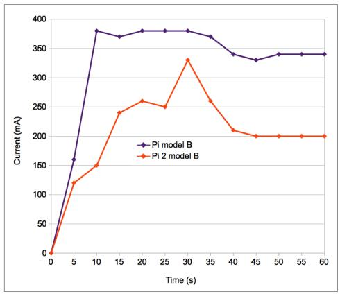
In Figure 1-3, I measure the current taken by a Raspberry Pi model B and compare it with a Raspberry Pi 2 model B.
