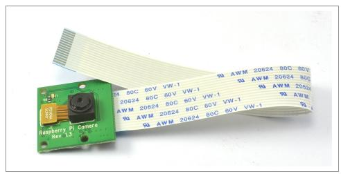
Figure 1-14. The Raspberry Pi camera module
