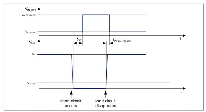
Figure 17 IN\_SET behavior during short circuit to GND condition with ST connected to GND and  $V_{\rm DEN}$  >  $V_{\rm DEN(act)}$
