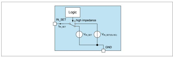
Figure 7 Block Diagram IN\_SET pin
