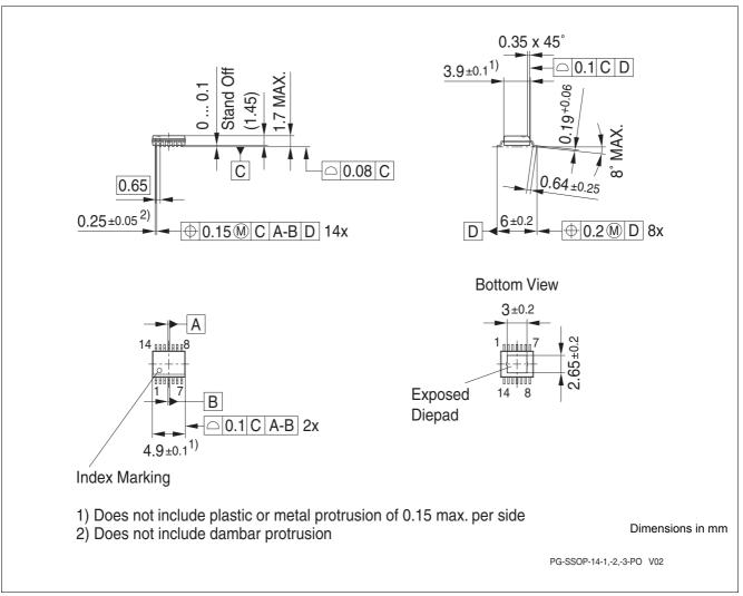
Figure 22 PG-SSOP14
