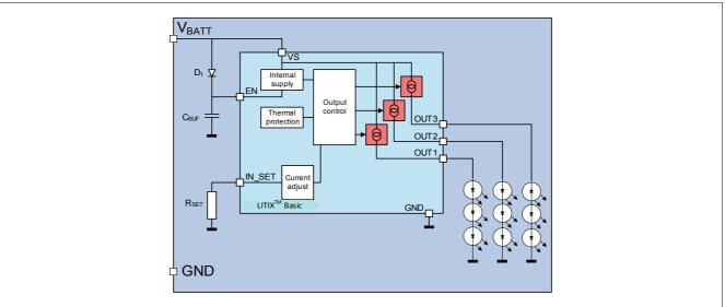
Figure 5 External circuit when applying a fast PWM signal on  $V_{\mathrm{BATT}}$
