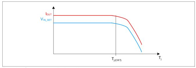
Figure 20 Output current reduction at high temperature
