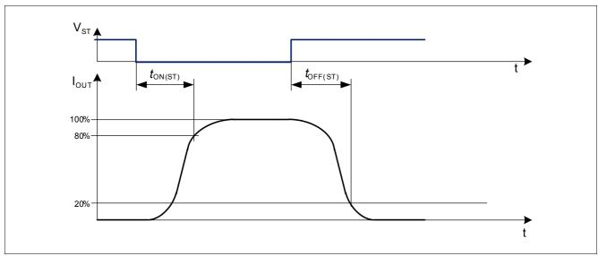
Figure 14 Switching times via ST Pin
