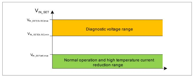
Figure 12 Voltage domains for IN\_SET pin, if ST pin is connected to GND
