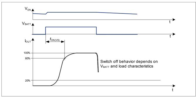
Figure 6 Typical waveforms when applying a fast PWM signal on  $V_{\mathsf{BATT}}$
