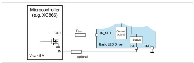
Figure 9 Schematics IN\_SET interface to  $\mu$ C, diagnosis via ST pin
