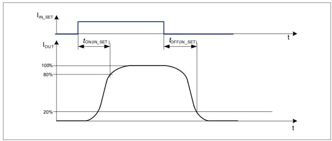
Figure 10 Switching times via IN\_SET
