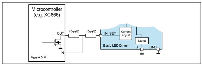
Figure 8 Schematics IN\_SET interface to μC, diagnosis via IN\_SET pin
