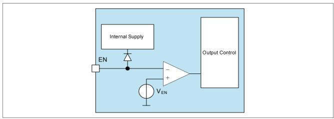
Figure 3 Block Diagram EN pin
