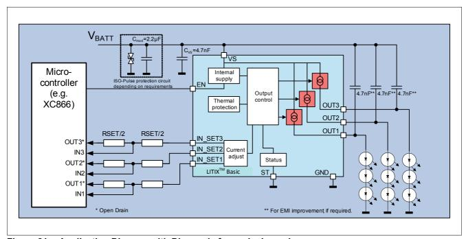
Figure 21 Application Diagram with Diagnosis for each channel
