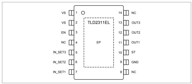
Figure 2 Pin Configuration
