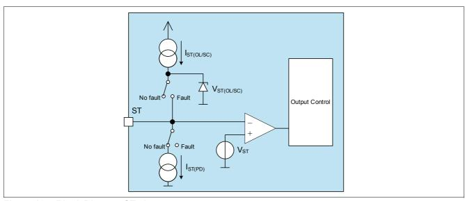
Figure 13 Block Diagram ST pin
