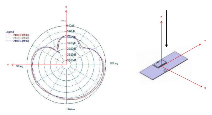
Figure 11: Radiation pattern of BLE121LR when mounted to a carrier board
