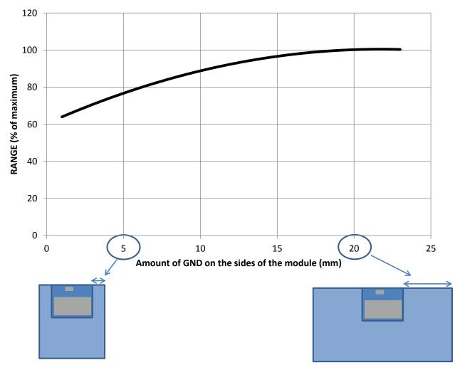
Figure 25: Impact of the size of GND plane to the range of BLE121LR
