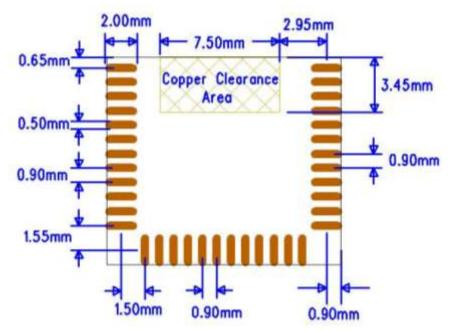
Figure 18: Recommended land pattern for BLE121LR-A
