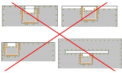
Figure 24: Poor layouts for BLE121LR
