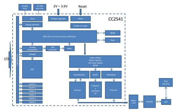
Figure 27: Simplified block diagram of BLE121LR
