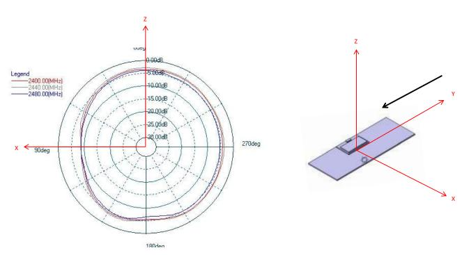
Figure 9: Radiation pattern of BLE121LR when mounted to a carrier board
