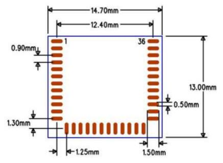
Figure 15: Footprint of BLE121LR (top view)
