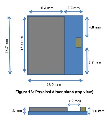
Figure 17: Physical dimensions (side view)
