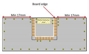
Figure 23: Recommended layout for BLE121LR-A
