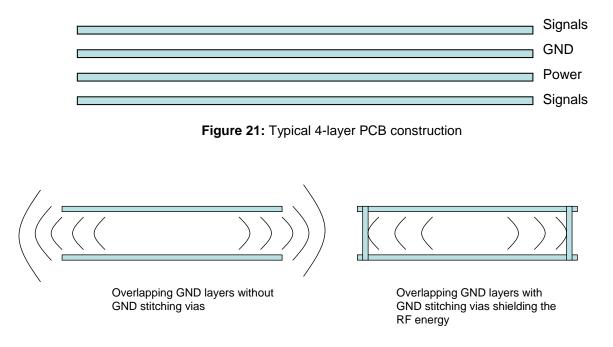
Figure 22: Use of stitching vias to avoid emissions from the edges of the PCB
