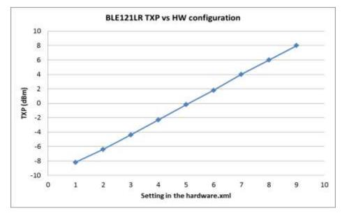
Figure 8: BLE121LR TX power as a function of the setting in the HW configuration file (Example: >>>>>>>>>>>>>>>>>>>>>>>>>>>>>>>>>>>>>>>>>>>>>>>>>>>>>>>>>>>>>>>>>>>>>>>>>>>>>>>>>>>>>>>>>>>>>>>>>>>>>>>>>>>>>>>>>>>>>>>>>>>>>>>>>>>>>>>>>>>>>>>>>>>>>>>>>>>>>>>>>>>>>>>>>>>>>>>>>>>>>>>>>>>>>>>>>>>>>>>>>>>>><tr<<td>>>>>>>><t
