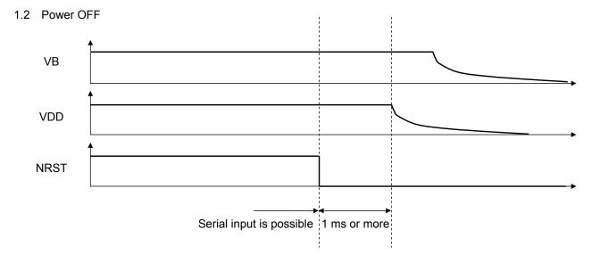
Note) Even if the power-off timing of VDD is the same as the falling timing of VB, there is no problem unless VDD voltage exceeds VB voltage.
