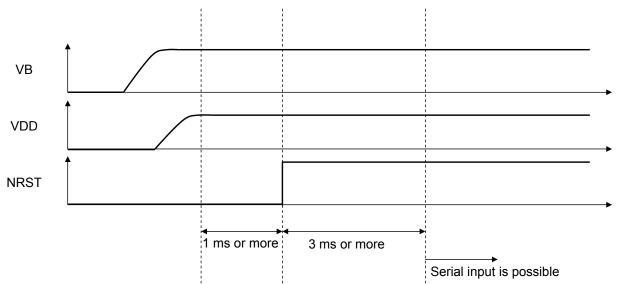
Note) Even if the power-on timing of VDD is the same as the rising timing of VB, there is no problem unless VDD voltage exceeds VB voltage.
