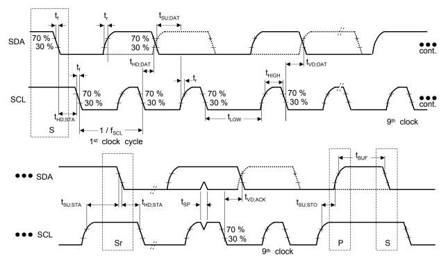
$V_{ILMAX} = 0.3_{VDD}$  $V_{IHMIN} = 0.7_{VDD}$
