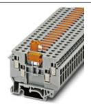
Knife disconnect terminal block, With test socket screws for insertion of test plugs, Connection method: Screw connection, Cross section: 0.2 mm² - 6 mm², AWG: 24 - 10, Nominal current: 16 A, Nominal voltage: 630 V, Length: 63.5 mm, Width: 6.2 mm, Color: red, Assembly: NS 35/7,5, NS 35/15, NS 32
