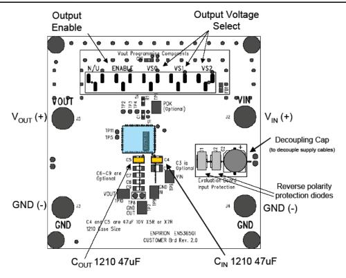
Figure 1. Evaluation Board Layout.
