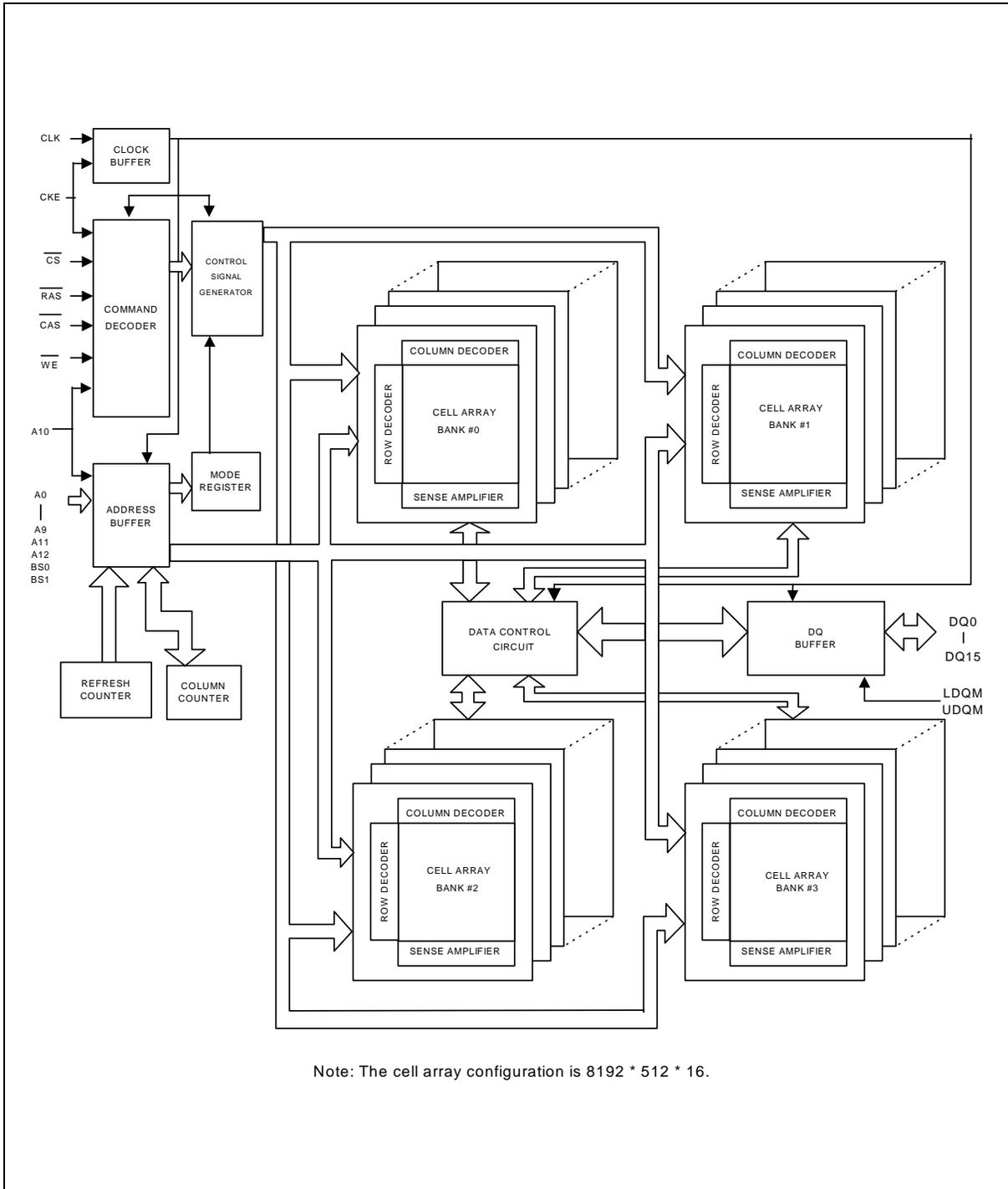
Note: The cell array configuration is 8192 \* 512 \* 16.
