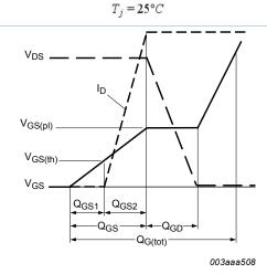
Fig. 12. Gate charge waveform definitions
