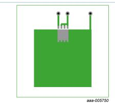
Fig. 5. PCB layout for thermal resistance junction to ambient 1" square pad; FR4 Board; 2oz copper
