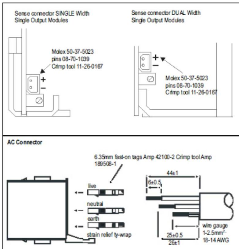
**S1 connector for single output modules**
