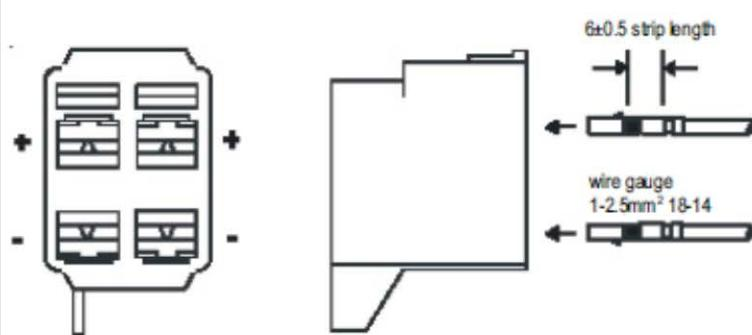
6.35mm fast-on tags Amp 42100-2 Crimp tool Amp 189508-1 max 25A per terminal, depending on wire.
