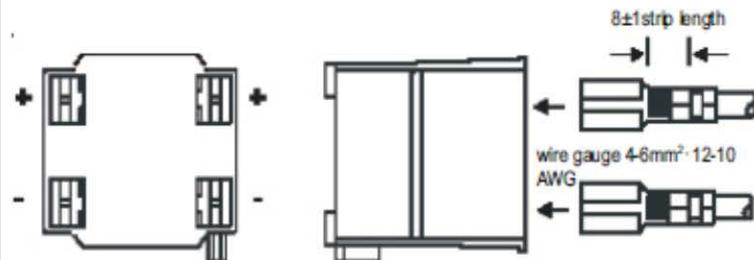
9.5mm fast-on tags Amp 151667-2 max 32A per terminal, depending on wire crimp tool Vogt3975C
