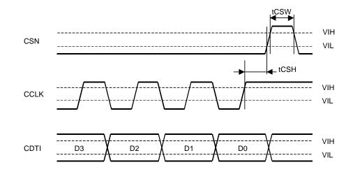
WRITE Data Input Timing (3-wire Serial mode)
