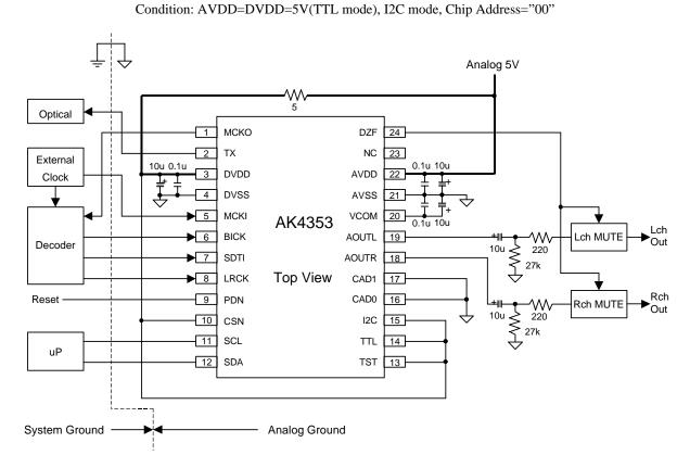
Figure 13. Typical Connection Diagram
