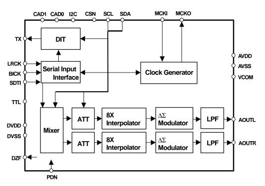
Figure 2.  $I^2C$  Bus Control Mode (I2C = "H")
