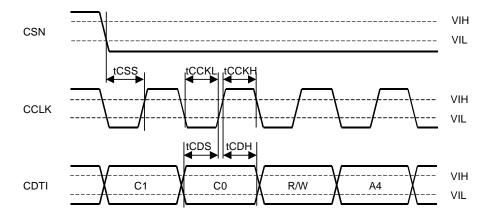
WRITE Command Input Timing (3-wire Serial mode)
