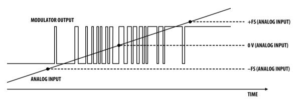
Figure 16. Modulator output vs. analog input.
