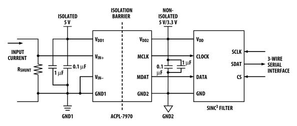
Note: In applications, 1  $\mu$ F/0.1  $\mu$ F bypass capacitors are recommended to connect between pins V<sub>DD1</sub> and GND1, and between pins V<sub>DD2</sub> and GND2 of the ACPL-7970.
