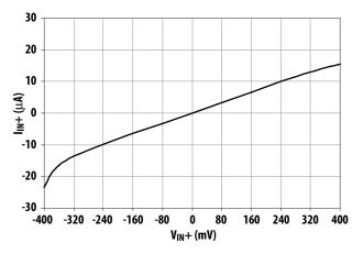
Figure 7. Input current vs. input voltage.
