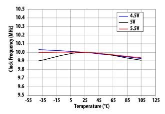
Figure 13. Clock frequency vs. temperature for various V<sub>DD1</sub>.
