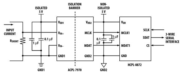
Figure 18. Typical application circuit with the HCPL-0872.
