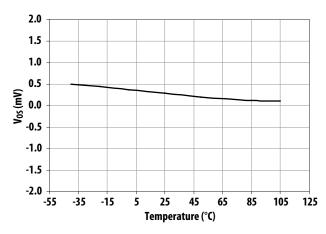
Figure 5. Offset change vs. temperature.
