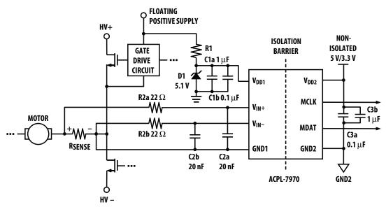
Figure 21. Schematic for three conductor shunt connection.
