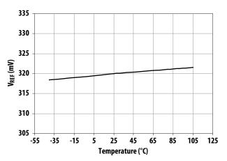
Figure 6. V<sub>REF</sub> change vs. temperature
