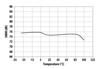
Figure 9. SNDR vs. temperature.
