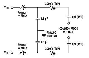
Figure 14. Analog input equivalent circuit.
