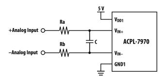
Figure 15. Simplified differential input connection diagram.
