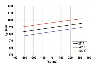
Figure 10.  $I_{\text{DD1}}$  vs.  $V_{\text{IN}}$  DC input at various temperatures.
