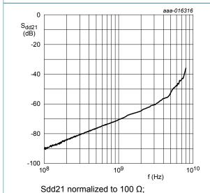
Fig. 3. Mixed-mode differential NEXT crosstalk; typical values
