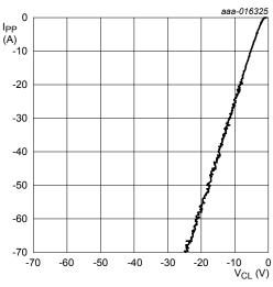
$t_p$  = 5 ns; Transmission Line Pulse (TLP);  $t_r$  = 600 ps
