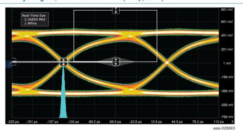
Test frequency: 148.5 MHz Differential swing voltage: 883 mV Horizontal scale: 34 ps/div
