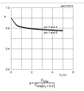
Fig. 2. Relative capacitance as a function of input voltage; typical values
