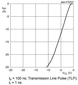
$t_r$  = 1 ns Fig. 10. Dynamic resistance with negative clamping;
