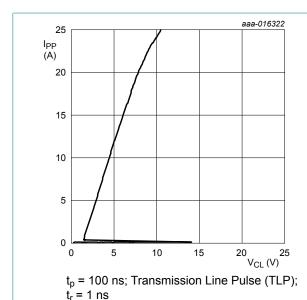
Fig. 9. Dynamic resistance with positive clamping; typical values
