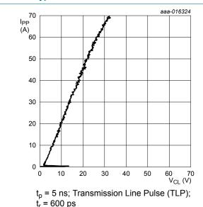
Fig. 11. Dynamic resistance with positive clamping; typical values
