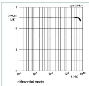
Fig. 1. Insertion loss; typical values
