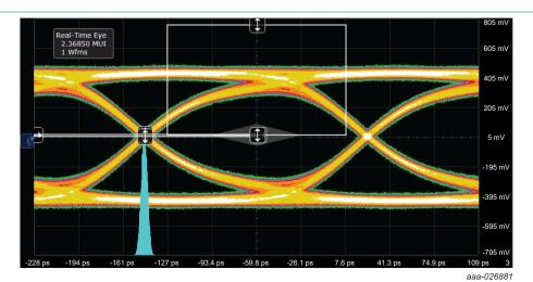
Test frequency: 148.5 MHz Differential swing voltage: 851 mV Horizontal scale: 34 ps/div
