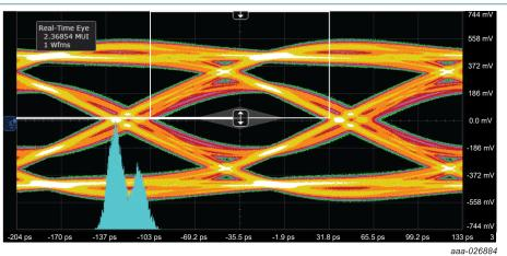
Test frequency: 148.5 MHz Differential swing voltage: 884 mV Horizontal scale: 34 ps/div
