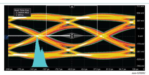
Test frequency: 148.5 MHz Differential swing voltage: 859 mV Horizontal scale: 34 ps/div
