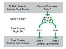
Figure 3. Example of code 5 broken into its binary components, which are code 4 and code 1.
