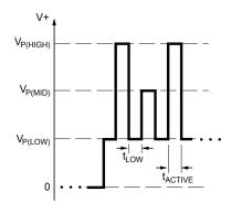
Figure 1. Parameter selection pulse train. This shows the sequence for selecting the register corresponding to key 1, indicated by a single  $V_{\text{PM}}$  pulse.
