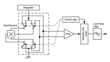
Concept of Chopper Stabilization Technique
