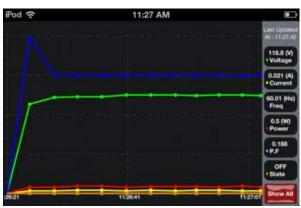
The Smartplug ADK works with the GainSpan Home Energy Management System (HEMS) ADK, which can be used to control multiple smartplugs and thermostats on the home network. The HEMS app allows selection and control of multiple devices, either one-at-a-time or all-together. Once device is selected, the app allows load on/off control as well as a graphical display of the power measurements.
