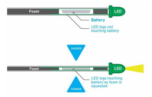
The torch works by powering a white LED from a coin cell battery. When the legs of the LED are touched against the terminals (faces) of the coin cell battery by squeezing the foam core, electricity flows from the battery through the LED, causing it to light up.
