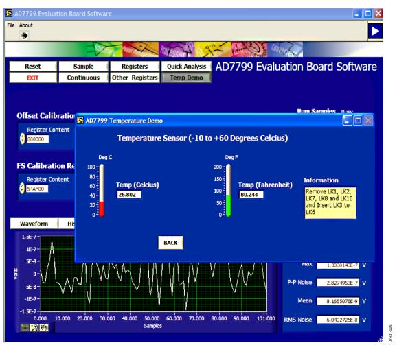
Figure 6. AD7799 Evaluation Software Temperature Demo Window
