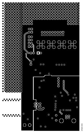
Figure 10. AD7799 Evaluation Board—Solder Side Artwork
