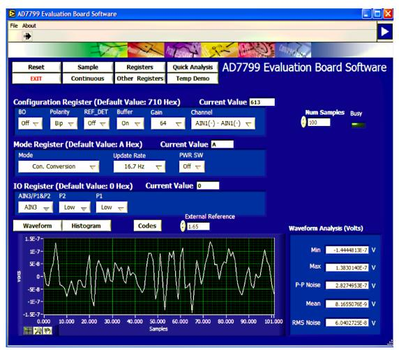
Figure 4. AD7799 Evaluation Software Registers Window
