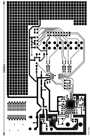
Figure 9. AD7799 Evaluation Board—Component Side Artwork
