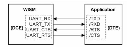
Port UART\_TX transmits data to the application's /RXD input.
