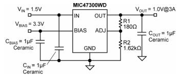
Figure 1. Typical Application Circuit
