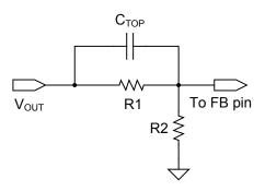
Figure 10 — Capacitor Coupling to FB Pin
