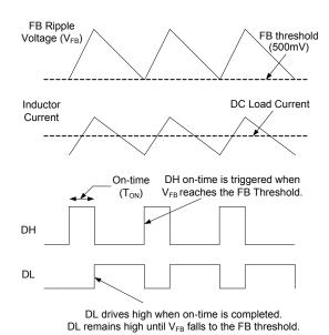
Figure 4 — Forced Continuous Mode Operation
