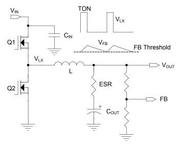
Figure 1 — PWM Control Method,  $V_{OUT}$  Ripple
