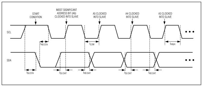
Figure 4. SMBus Serial Interface Timing—Address
