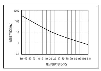
Figure 9. Typical Thermistor Characteristics
