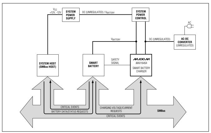
Figure 10. Typical Single Smart Battery System
