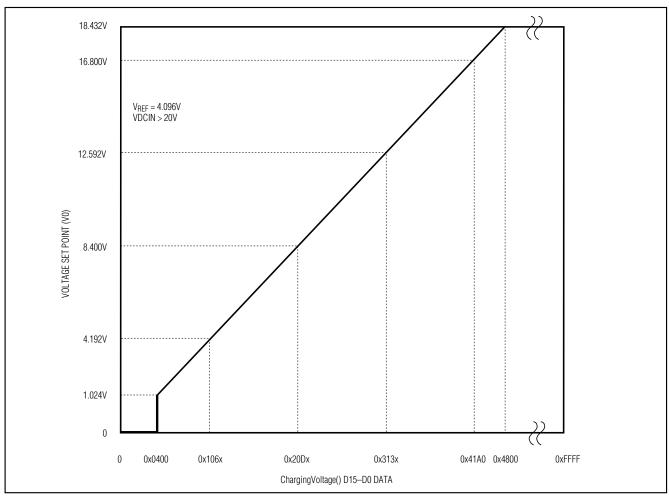
Figure 7. ChargingVoltage() Code to Voltage Mapping
