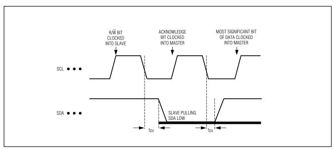
Figure 5. SMBus Serial Interface Timing—Acknowledgment
