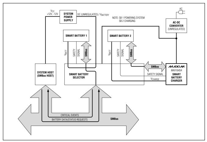
Figure 11. Typical System Using Multiple Smart Batteries
