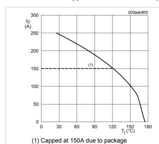
Fig. 1. Continuous drain current as a function of mounting base temperature
