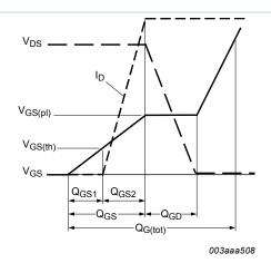
Fig. 13. Gate charge waveform definitions
