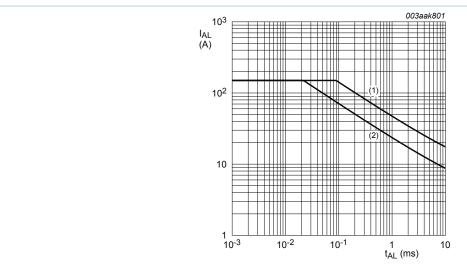
Fig. 3. Avalanche rating; avalanche current as a function of avalanche time
