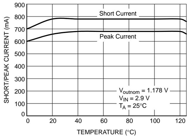
Figure 7. Peak and Short Current vs. Temperature
