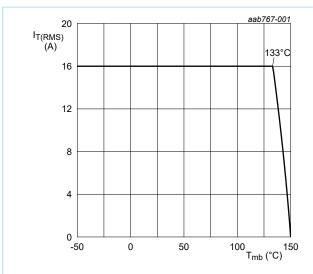
Fig. 2. RMS on-state current as a function of mounting base temperature; maximum values
