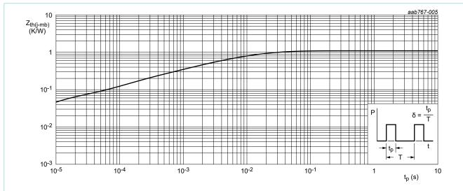
Fig. 6. Transient thermal impedance from junction to mounting base as a function of pulse duration
