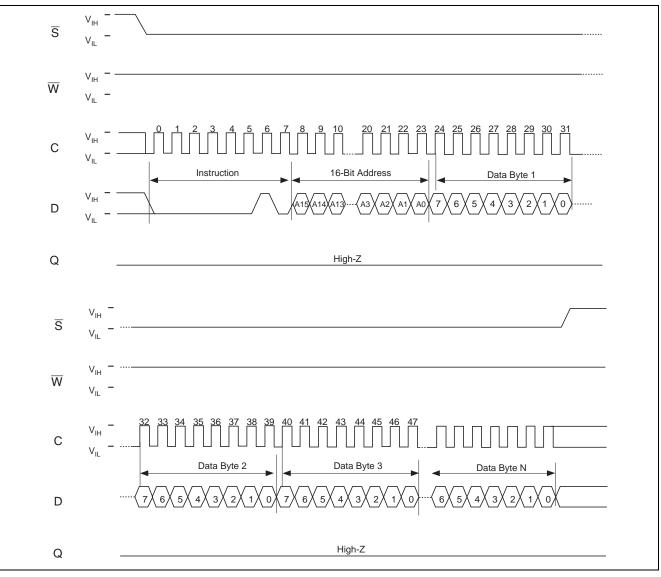
Note: 1. Depending on the memory size, as shown in Address Range Bits table, the most significant address bits are don't care.
