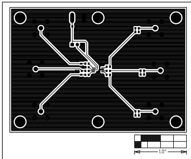
Figure 3. MAX9653 EV Kit PCB Layout—Component Side
