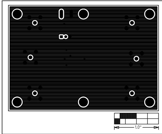
Figure 4. MAX9653 EV Kit PCB Layout—Solder Side
