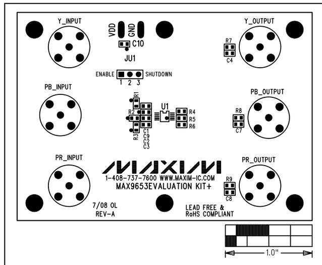
Figure 2. MAX9653 EV Kit Component Placement Guide—Component Side
