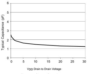
Figure 7. Output Capacitance
