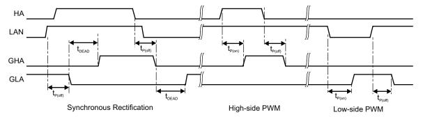
Figure 3a: Gate Drive Timing – Phase A Logic Control Inputs
