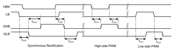
Figure 3b: Gate Drive Timing – Phase B Logic Control Inputs
