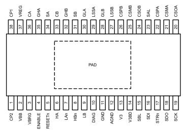
Package LP, 38-Pin eTSSOP Pinout Diagram
