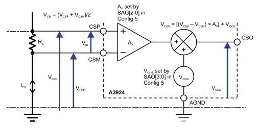
Figure 12: Typical Sense Amp Voltage Definitions
