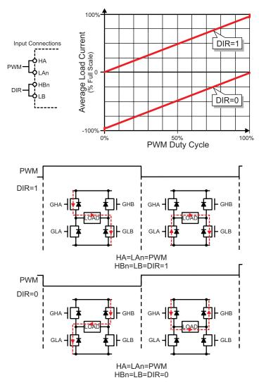
Figure 9: PWM and DIR Inputs, Slow Decay, SR
