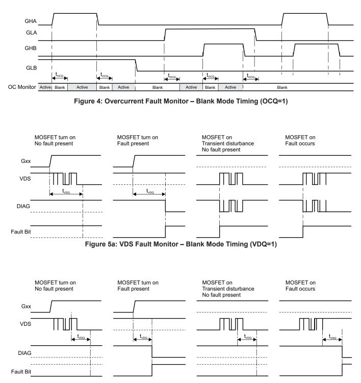
Figure 5b: VDS Fault Monitor – Debounce Mode Timing (VDQ=0)
