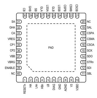
Package EV, 40-Pin eQFN Pinout Diagram
