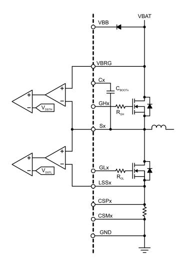
Figure 7: VDS Overvoltage Fault Detection
