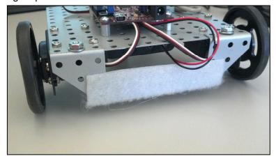
14. Cut four ½-inch sections of Velcro from the other 4-inch strip. Attach these 1/2 –inch strips to each of the four IROS sensors.
