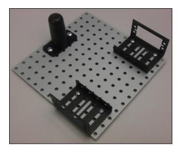
3. Add the standoffs to the robotic kit as shown below. Set four extra screws aside to mount the MX3cK in a later step.
