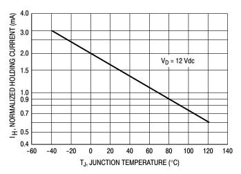
Figure 5. Typical Holding Current versus Temperature
