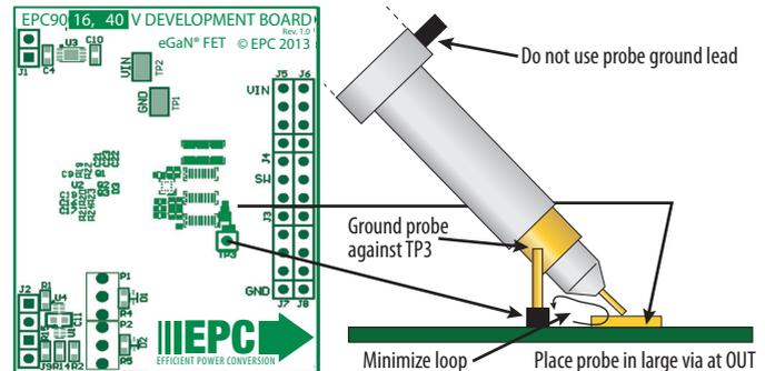
Figure 3: Proper Measurement of Switch Node –  $V_{SW}$
