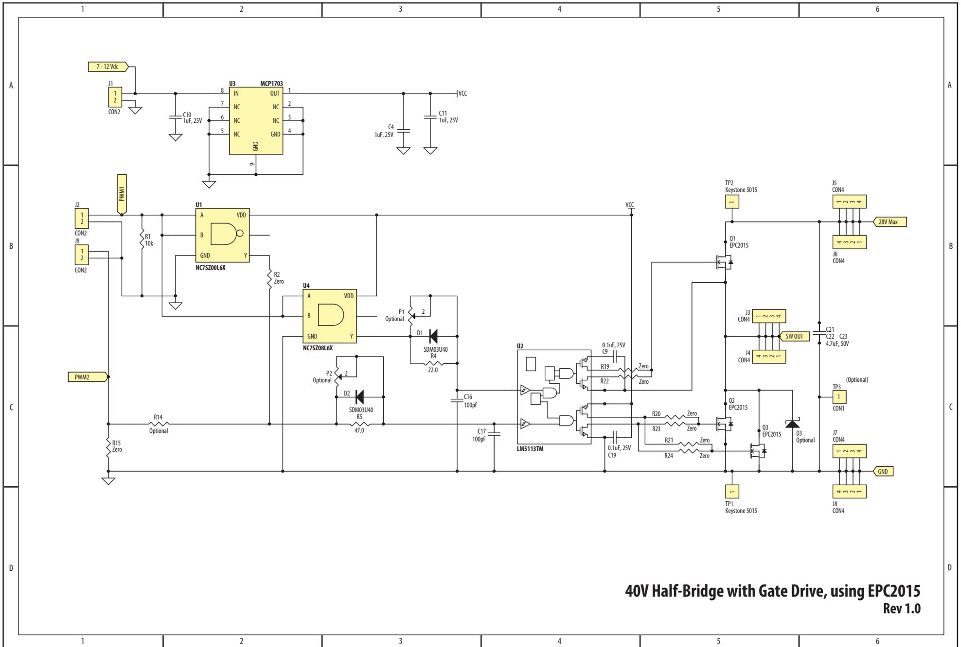
**40V Half-Bridge with Gate Drive, using EPC2015**
