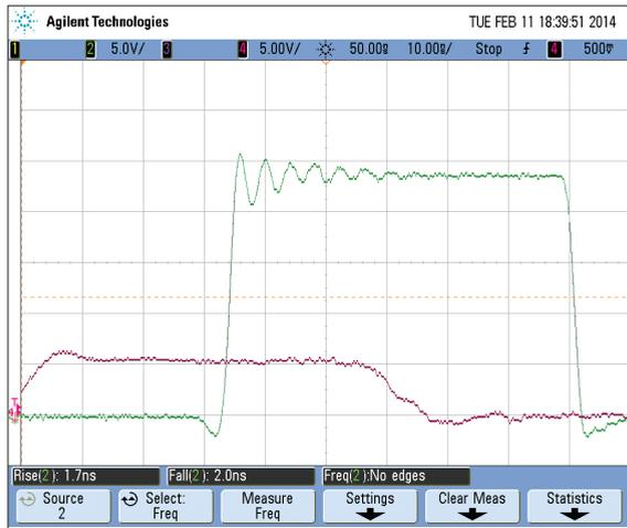
Figure 4: Typical Waveforms for  $V_{IN} = 24\text{ V}$  to  $1.2\text{ V}/25\text{ A}$  (1000kHz) Buck converter
