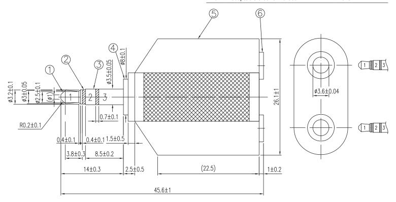
Ø3.5 Stereo Plug Ø3.5 Stereo Receptacle Schematic
