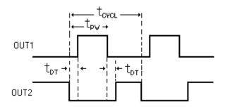
Figure 4: Output Waveform Displaying Dead-Time
