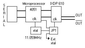
Figure 2 - EVDP610 Functional Block Diagram
