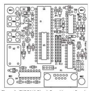
Figure 8 - EVDP610 Circuit Board Layout Drawing
